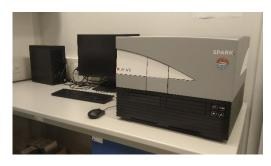
Another addition to the facility is a Spark microplate reader which offers absorbance (from 200 to 1 000 nm), fluorescence, including FRET and fluorescence polarization, and luminescence (ex 230 – 900 nm, em 280 – 900 nm) measurements. This technique provides a solution for ELISAs, low volume DNA/protein quantification and fast spectral scanning. It offers cuvettes and microplate formats up to 1536 wells, has a higher performance, sensitivity and flexibility.
