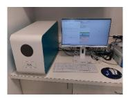
The CF was supplied with the new SpectroLight 600 for measurement of dynamic light scattering in drops (including crystallisation experiments). Detection of suitability of samples for crystallization or CryoEM grid preparation, together with in situ time lapse monitoring of protein crystallization and detection of nanocrystals for electron diffraction.
