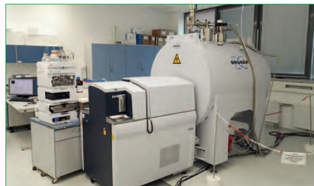
Bruker Daltonics 15T-Solarix XR FT-ICR ultra-high resolution mass spectrometer at the CMS, with electrospray and MALDI ion sources, coupled to an Agilent Technologies 1200 HPLC system.
