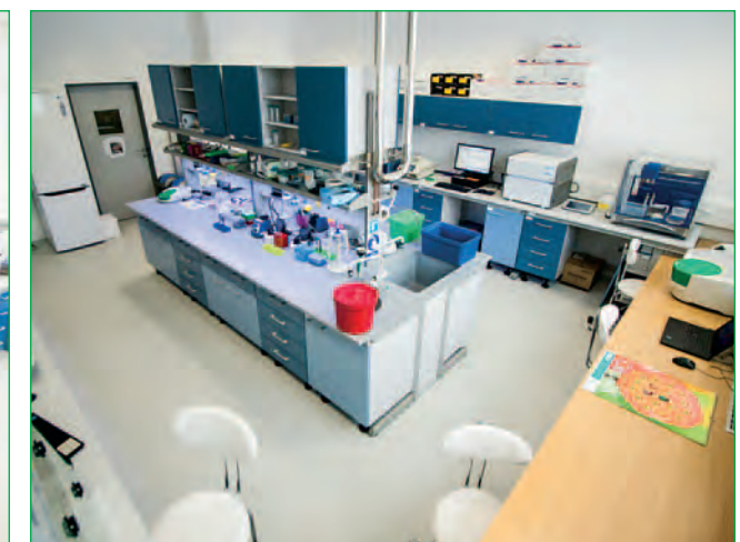
Core facility Genecore and its equipment for nucleic acid analysis including BioMark, loading stations, qPCR instruments and robotic liquid handling
