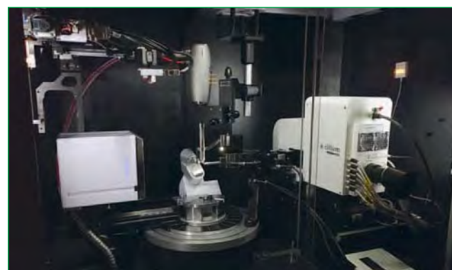
Bruker D8 Venture diffractometer with a high-flux liquid Gallium MetalJet D2 X-ray source, Photon II detector and Kappa goniometer. This is also equipped with an ISX motorized stage for in-situ X-ray diffraction experiments, enabling screening of diffraction properties in crystallization trays.
