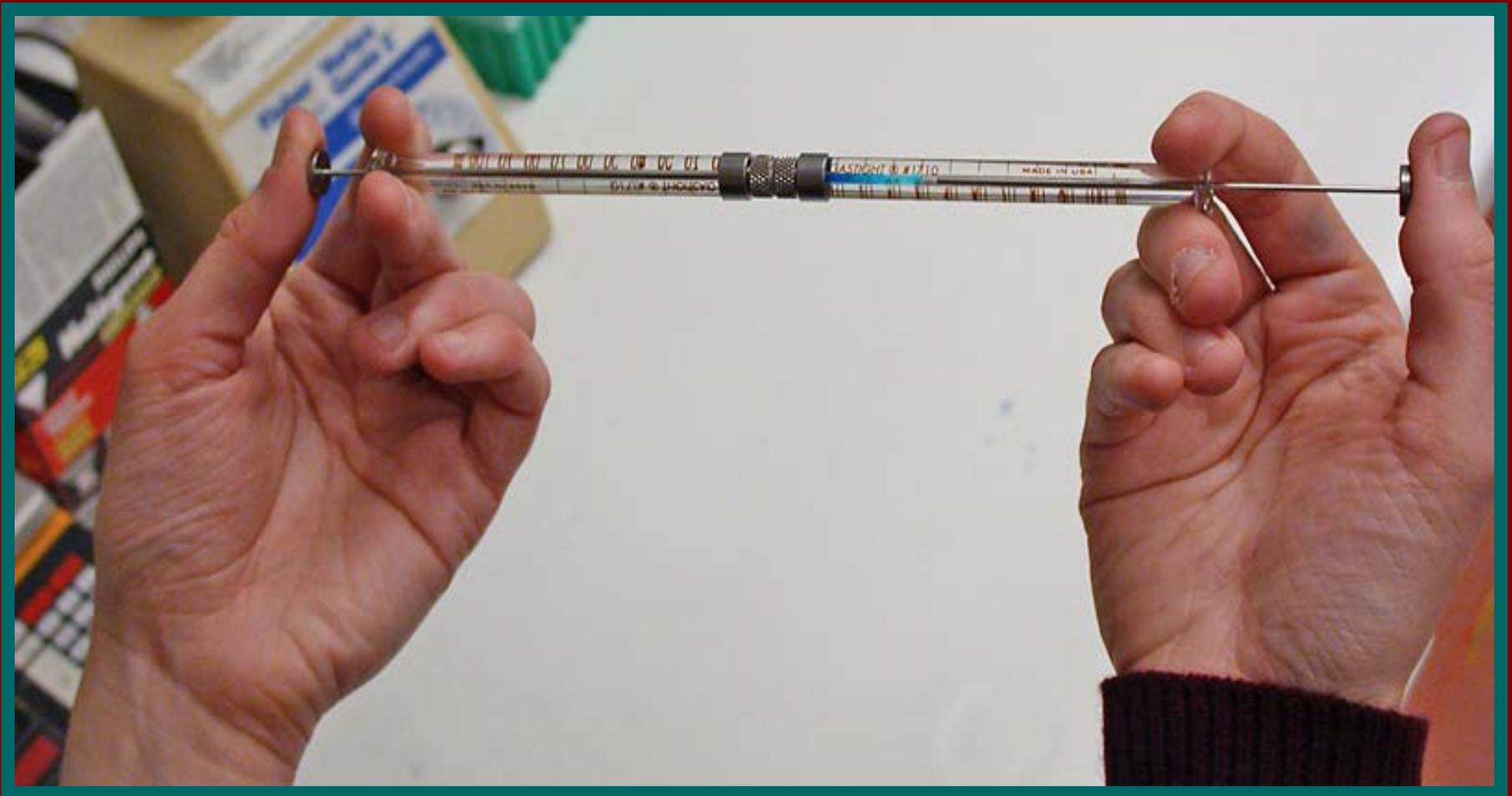
**Mechanically mixing the protein solution and lipid together to form the cubic mesophase**
